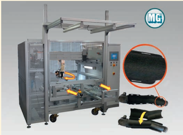
Fixing of acoustic capsules to plastic pipes
