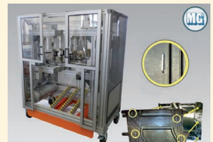
Attachment of aluminium sheets onto plastic panels
